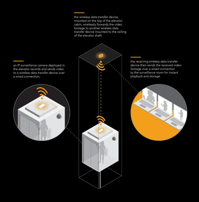
This can be done with wireless devices mounted to the bottom of the elevator cabin and the ground platform of the shaft, if necessary. There is also the option of setting up links on both sides of the elevator cabin, one serving as the main and the other as the redundancy link.
